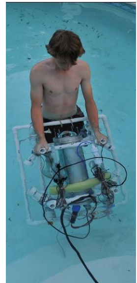
ROV's natural tilted position before balancing
